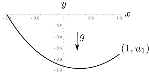
Figure 6.1: the shape of a chain hanging from its endpoints in gravity
