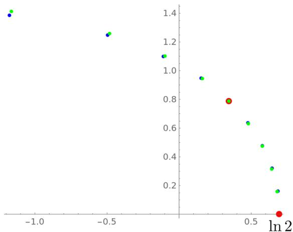
Figure 1: The points for  $f(0)$  and  $f(e^{i\pi/4})$  are computed with 100,001 terms of the series and are shown in red. The points in blue are computed with 101 terms of the series, and the points in green are computed with 1001 terms. As you can see, there is not much movement from the blue to the green to the red, so we probably have a reasonable numerical representation of the values.
